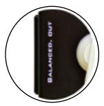
Balanced XLR output (200 ohm) for direct recording or PA (Not digital audio). PLEASE NOTE when using this output does the AUX input not work, nor the master volume. In this mode ONLY guitar the input, and amp/speaker simulator are active. The volume is set on the guitar knob, please be aware not overloading the mixing consol input.
