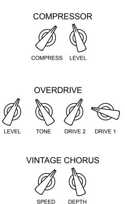
**Compressor:** Compression is a very good effect for overall use, it smoothes out your uneven dynamics, increases sub tones which otherwise would stay too weak in the overall sound. It also gives more depth, body and sustain for a fuller sound. This is great for especially solos. Just set the level knob to match the desired solo level. For more compression turn the compress knob clockwise, and adjust your level to match the bypass level.
