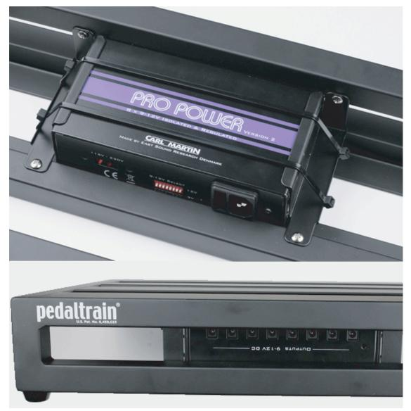
The bonus is you now can get to the DC out's very easy, while the mains power cord is inside under the board good and safe, the mains and voltage switches is also inside the board. Elegant, neat and very sturdy.
