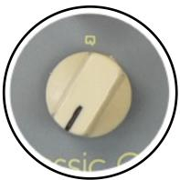
The Q knob adjusts the bandwidth for the Classical Optical Envelope. At full counter clockwise you have a very wide bandwidth which provides you with a soft, round and warm wah effect. At full clockwise, the opposite is true....the bandwidth is very narrow and provides you with a sharp, ear-ripping effect. The setting of the Q knob is very interactive with both the Drive and Tone knobs, and you may find that you have to adjust the Level as well, depending on your other settings.
