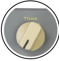
The Tone knob on the Classic Optical Envelope, is a high cut filter. With the knob set at full clockwise, you enjoy the full bandwidth of frequencies, so as you turn the knob counter clockwise, you start to filter out the high frequencies. On this effect, the Tone control works interactively with the Drive control, so as you adjust the Drive, you may find that you have to 'tweak' the Tone control to achieve your optimum tone.
