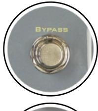
Our Bypass button on the Classic Optical Envelope simply switches the effect on and off. This is a high quality buffered bypass (NOT True Bypass) which ensures silent switching and no loss of high frequencies due to long cables or multiple pedals....a critical feature for envelope filters which rely on full bandwidth.
