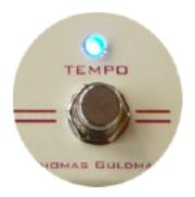
With the TAP TEMPO chosen on the select switch LED on, you can set the delay time simply by tapping the desired or the song tempo on the TEMPO switch with your foot, you shall tap minimum two times ore more as the unit will always set the tempo after the last two tap's.
