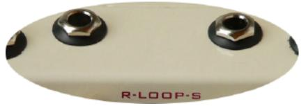
With the LOOP you can insert an external effect device, i.e. a Chorus or Phase, even an overdrive pedal or EQ with this you can either color or modulate the echo in a ton of different ways with really cool results. But please notice the effects in the loop only work on the repeats not the overall main guitar tone.
