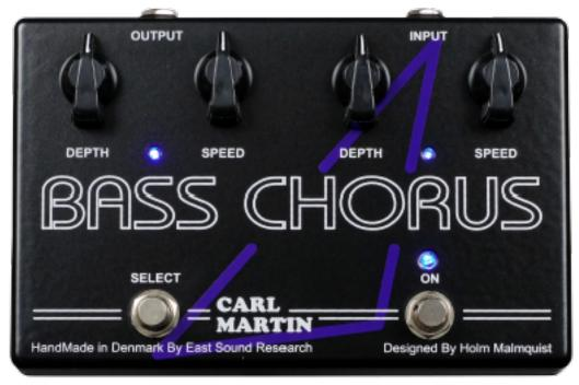
Although similar in function to the older Chorus XII, it is housed in the new wider/lower metal housing with 'chicken-head knobs' for adjustment. Of course, the quality remains the same, and the new housing also encloses the regulated +/-12V power supply for maximum headroom and clarity.
