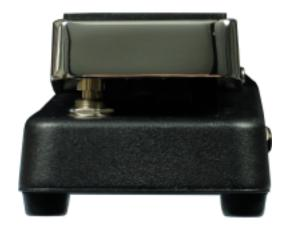
By stepping on the back of the rocker you engage the Mode switch, between low and high mode.
