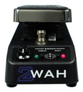
The standard effect on-off by stepping on the front of the rocker to engage the true bypass on-off switch.
